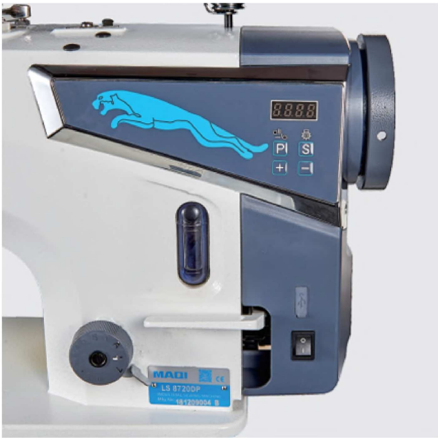
Self-produced electronic control, intelligent USB port
